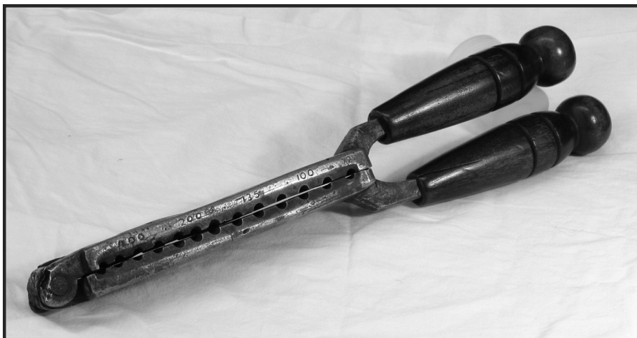
The hinged mold is made of brass with handles carved from cherry wood. Liquefied metal was poured into the various sized holes for shaping into shot and bullets.
